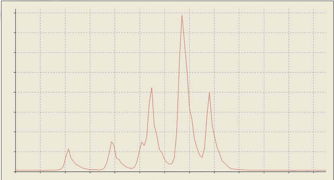
Figure 4 Measurement of an 850 nm optical transceiver with a high-end standard spectrometer.
